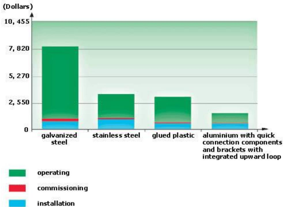
Technologies offering smooth bore pipe work (aluminum, plastic) provide a high reduction in pressure drop and thus also operating costs. Conversely galvanized steel systems, affected by rust and pitted interior surfaces after several years of use, cause higher operating costs.
