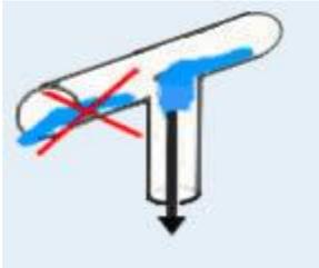
Condensate collects within the pipeline and circulates throughout the system.
