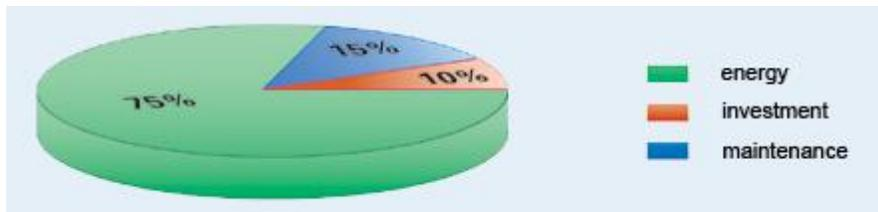
The pie chart above illustrates the typical cost breakdown for an average compressed air system (compressor, pipe system, and operating costs) over a 10 year period.
