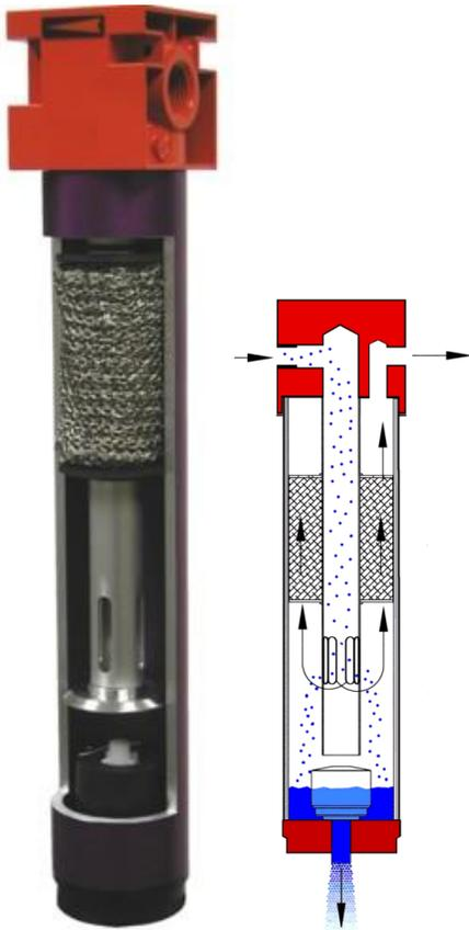
Air enters the unit and goes down through the center tube. Moisture then gathers in the bottom bowl to be drained while the dry air goes back up and exits the unit.
