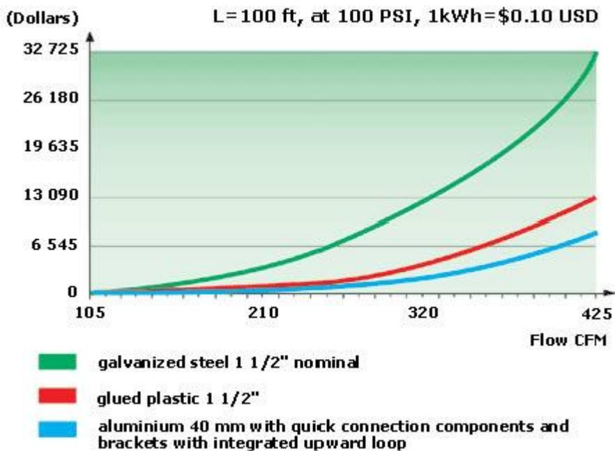
Technologies offering smooth bore pipe work (aluminum, plastic) provide a high reduction in pressure drop and thus also operating costs. Conversely galvanized steel systems, affected by rust and pitted interior surfaces after several years of use, result in higher operating costs.
