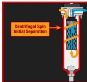
The water traps remove liquid already condensed in the airline. Aftercoolers and refrigerated dryers reduce the air temperature to a low dew point where the water vapor condenses and is removed before being distributed to the shop plumbing for use by the technicians.
